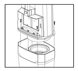
In order to disassemble the vac motor housing, remove the dust bag cover, unhook the vent grid and unscrew the four screws from the shell.
