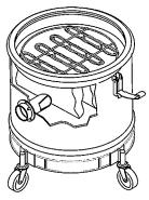
1) When installing the cloth filter assembly, the flat side of the cloth must sit in the tank as shown above so it does not interfere with the tank inlet.
