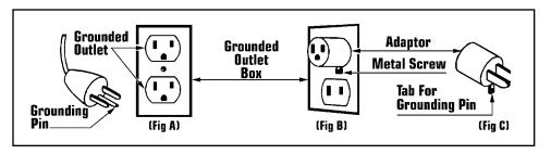
This electric equipment is for use on a nominal 120 volt circuit, and has a grounded plug that looks like the plug illustrated in (Fig A). A temporary adaptor that looks like the adaptor illustrated in (Fig B & C) may be used to connect this plug to a 2-pole receptacle as shown in (Fig B) if a properly grounded outlet is not available.
