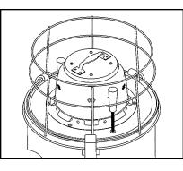
1) Position the hose cage on the motor head making sure the power cord is through the raised loop at the bottom of the cage.
