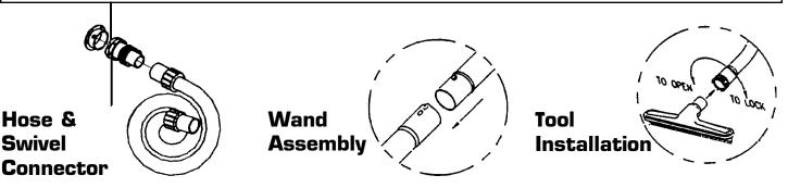
The hose and swivel connector are preassembled at the factory. To attach the swivel connector to intake fitting on the vacuum tank:
