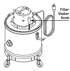
The filter shaker is designed to keep the cloth filter from clogging. When loss of suction occurs or every 30 minutes you need to use the filter shaker.
