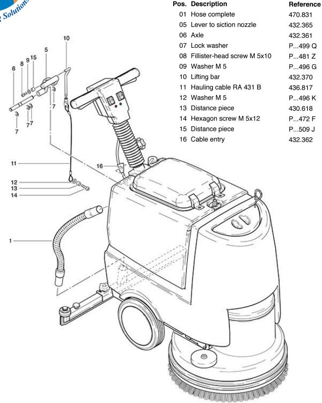
SD-17B 17-Inch Single Brush, Battery Powered Autoscrubber Angled Tube Drawing
