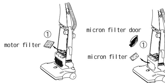
1. Open micron filter door, grasp micron filter and pull out.
