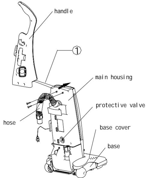
1. From rear of cleaner, align handle with groove and slide onto cleaner. If necessary, use thumb and finger pressure to slide handle into position.
