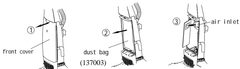
1. Remove front cover. Grasp both sides of bag cover near top. Push thumbs against center of cover and pull out on sides.
