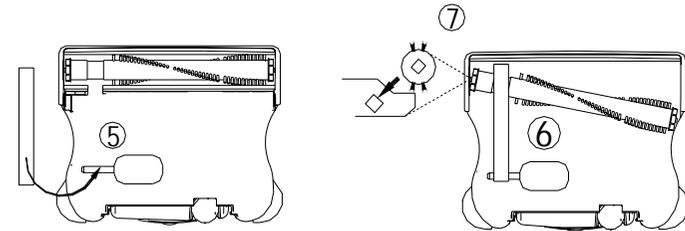
5. Place new belt around motor pulley.
