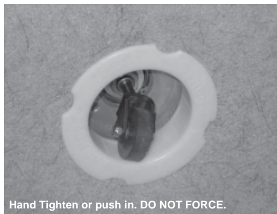
Install 20 Inch Pad inside pad driver. Hand Tighten center clip or push straight in.
