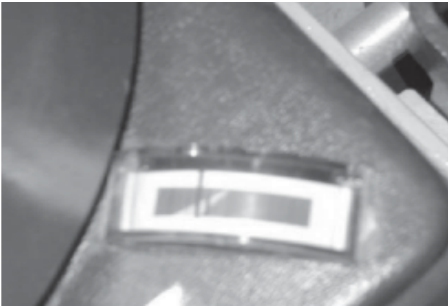
Pad Pressure Gauge. Needle will “peg” then drop to its normal pressure. Adjust pad pressure knob so pad pressure gauge reads at the 15 amp red line. Be sure to keep unit moving to prevent damage to the floor.
