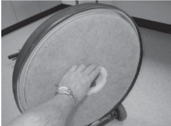
Install 20 Inch Pad inside pad driver. Hand Tighten center clip or push straight in.
