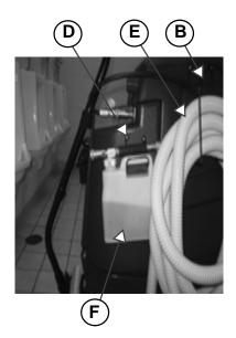
Left hand side large bracket will hold the recovery hose. Small bracket holds chemical proportioning tank.
