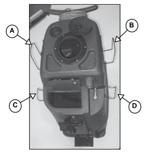
The unit is equipped with 4 wire brackets two small and two large
