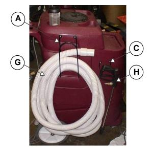
Right hand side large bracket will hold the blower hose. Right hand side small bracket will hold the pressure gun.
