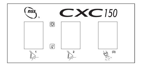
**VACUUM SWITCH (1 & 2):** Each switch turns on one vac motor. Turn both switches on for maximum lift. The vac switches illuminate when turned on.
