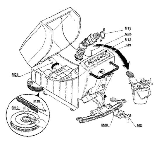
**Squeegee:** Every week, check the blades of the squeegee and wash them carefully. Then replace them in the correct working position *(see above)*. If drying is not perfect even after the unit has been cleaned, replace any blades which are excessively worn. If the squeegee does not pick up enough water or streaks, lift and wipe off the blades. Inspect the squeegee vacuum path for obstructions.
