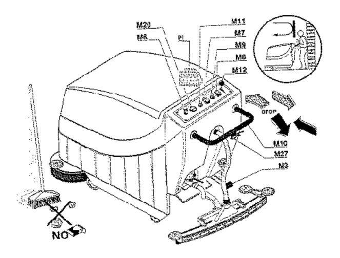
The area to be scrubbed: Debris and grit must be swept up before starting the scrubbing operation to avoid vacuum line blockage and to permit the detergent to perform efficiently.
