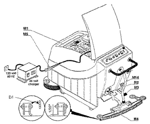
**Solution Tank:** The solution tank is located under the lid, at the front of the machine, with the filling-funnel **M1** in an accessible position for easy re-filling.
