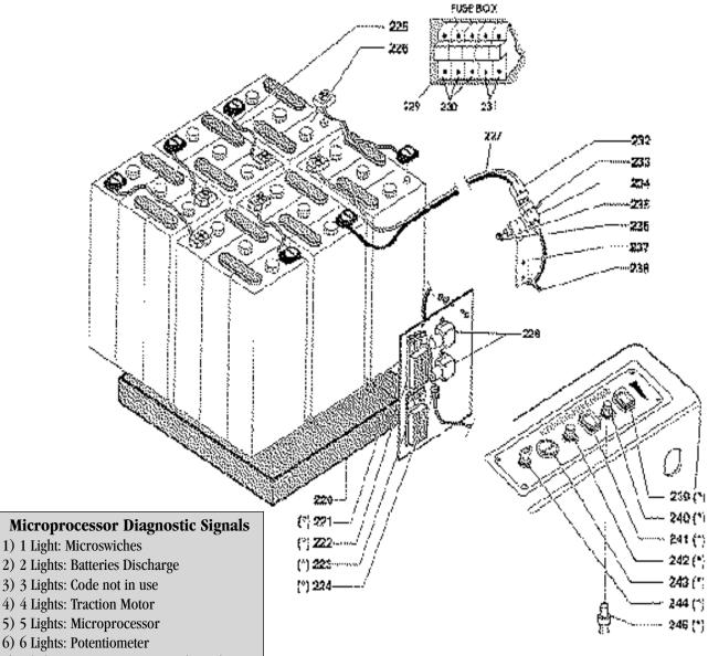
2) 2 Lights: Batteries Discharge 3) 3 Lights: Code not in use 4) 4 Lights: Traction Motor 5) 5 Lights: Microprocessor 6) 6 Lights: Potentiometer
