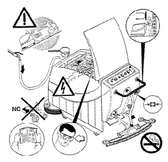
WARNING! Do not operate machine or charger in areas where flammable liquids or gases are present. Do not use or pick up flammable chemicals or liquids with this machine.
