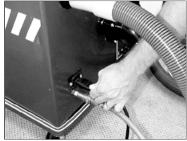
Connect the male power cord plug to the cordset adaptor and the cordset adaptor to the Powr-Extractor Brush receptacle on extractor.
