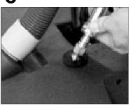
Attach the solution hose female connector to the male connector located on top of the Powr-Extractor Brush housing.
