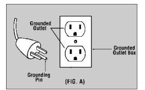
This unit is for use on a nominal 120 volt circuit and has a grounded plug that looks like the plug illustrated in (Fig. A).
