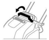
2. Lift upper recovery tank from machine and set aside.
