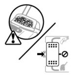
6. Empty recovery tank when approximately 3/4 full. If the recovery tank is overfilled, the water will drain back onto the carpet when the vacuum is switched off.
