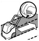
5. While operating machine, check for excessive foam buildup in the recovery tank. If excessive foam is present, add a defoamer solution to recovery tank, or empty tank.
