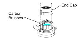
If armature commutator is grooved, extremely pitted or not concentric, the motor will need to be replaced or sent to a qualified service center.
