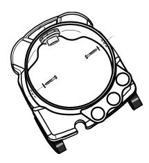
5. Place the handle over the two ends of the screws.
